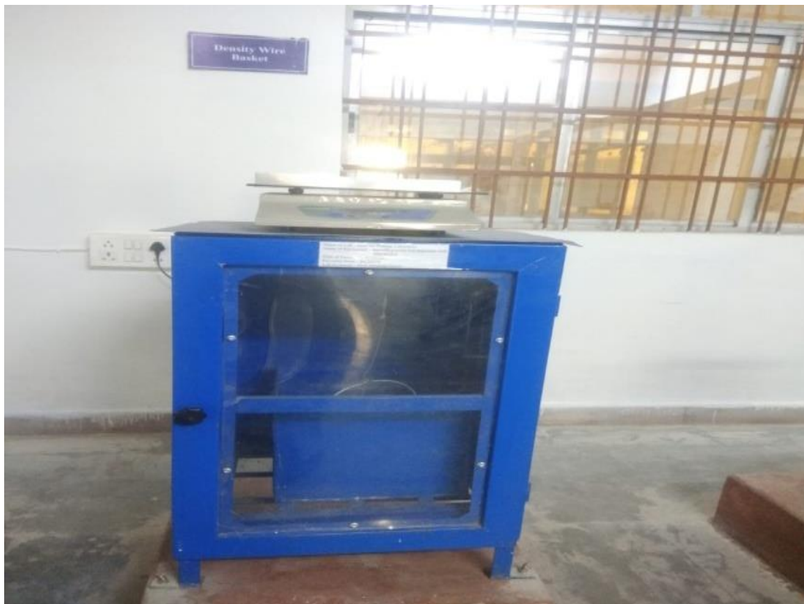
Figure 1h. Specific Gravity & Water absorption test machine of coarse aggregate
