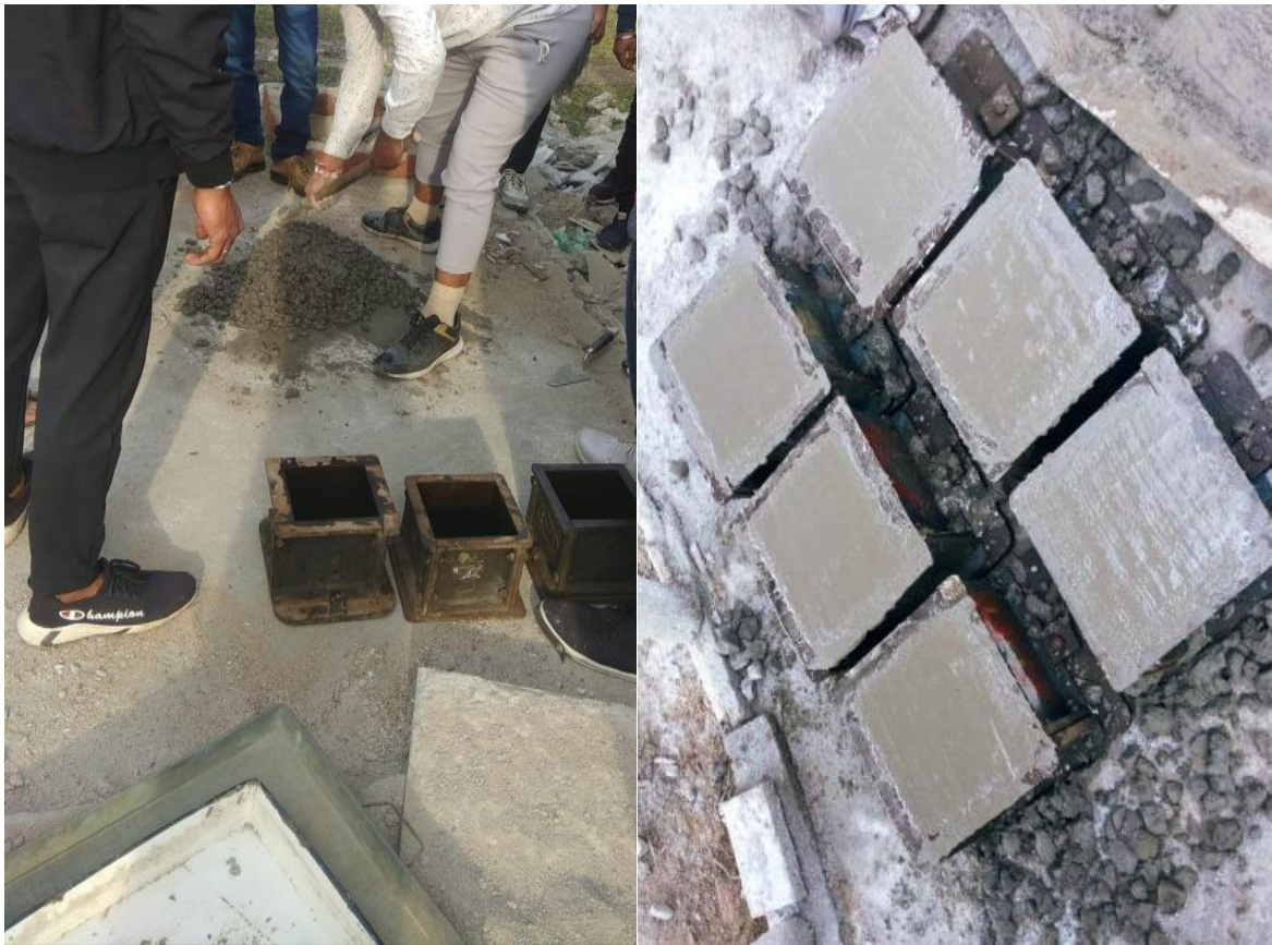
Figure 1i. Casting of cubes
