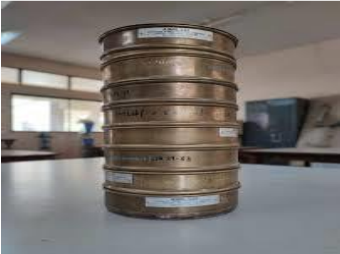
Figure 1g. Sieve analysis of sand
