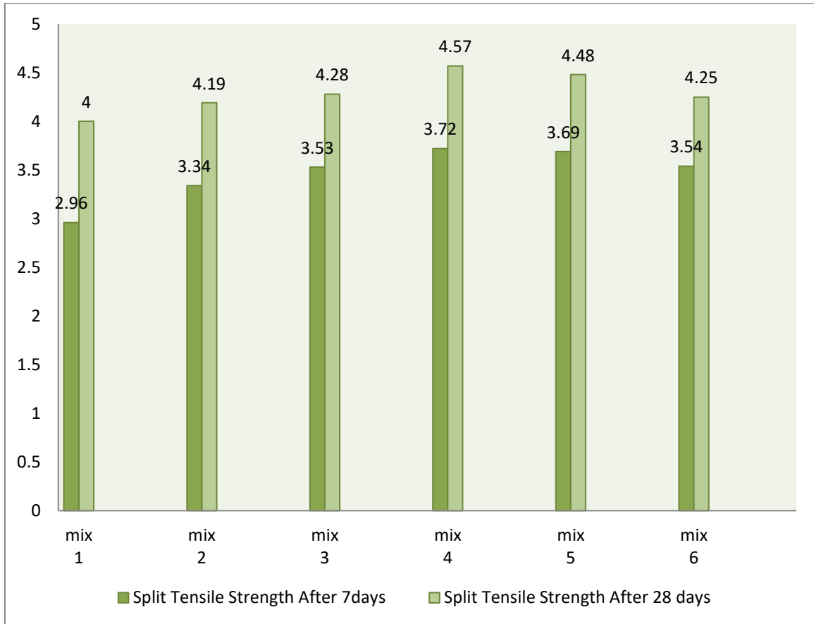
Figure 2d. Result of Split Tensile Strength Test of M40 Grade concrete
