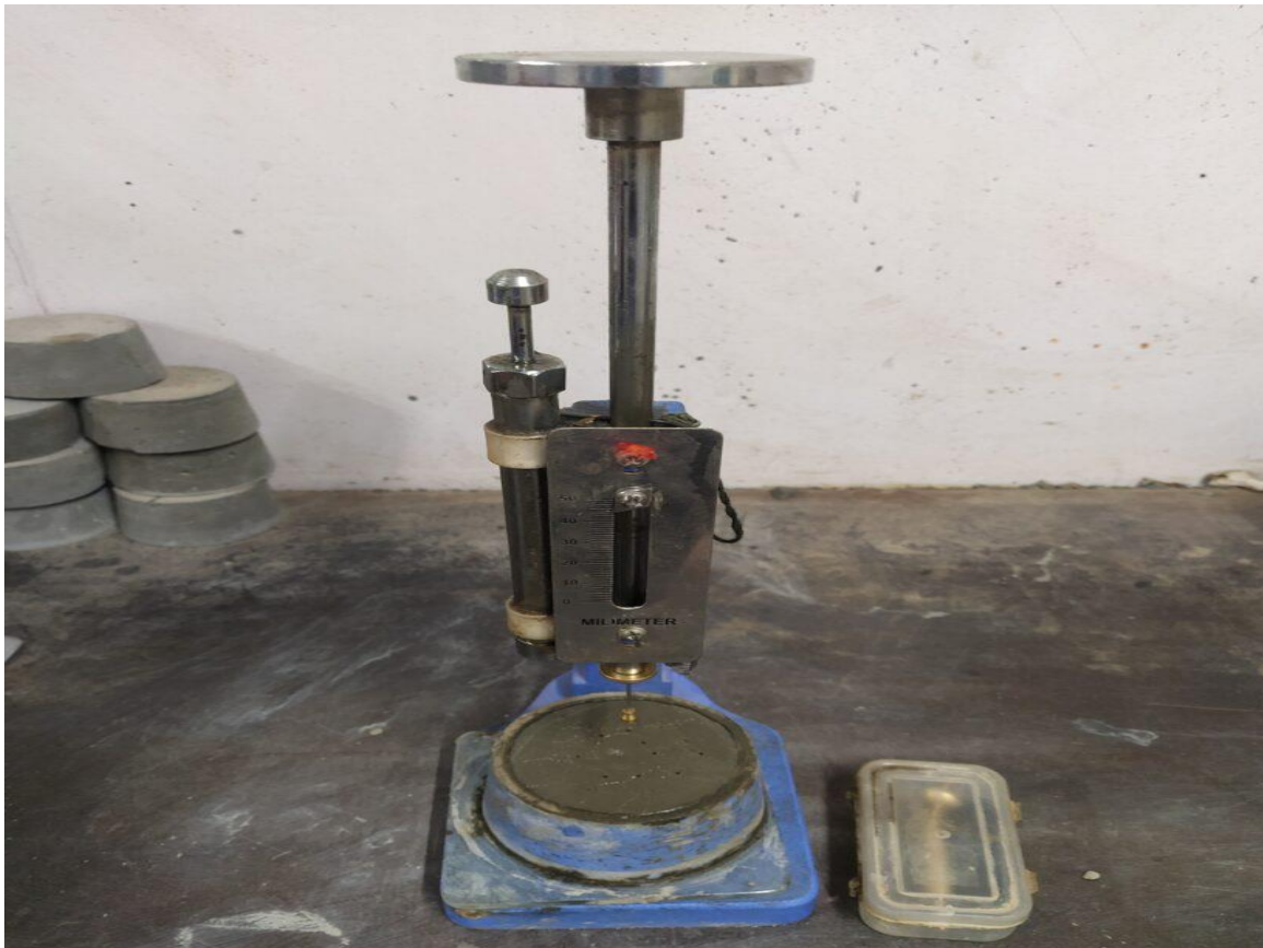
Figure 1e. Vicat Apparatus for Consistency, Initial setting time & Final setting time test of cement
