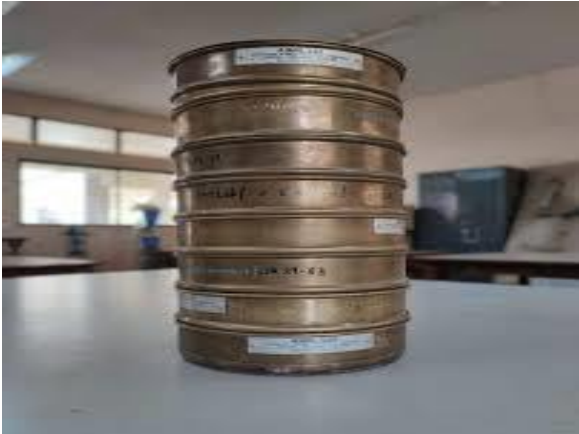
Figure 1g. Sieve analysis of sand
