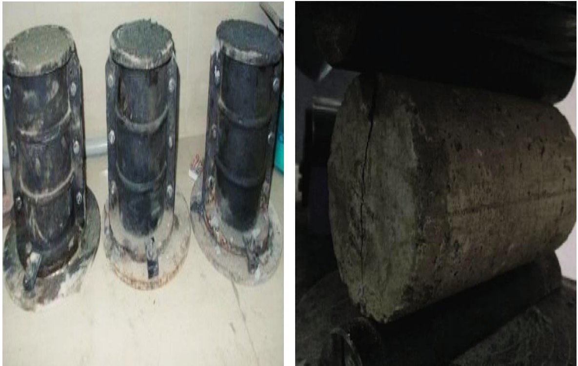
Figure 1k. Split Tensile Strength test of Concrete Cylinder by CTM machine
